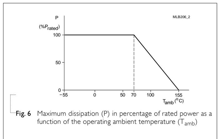
Fig. 6 Maximum dissipation (P) in percentage of rated power as a function of the operating ambient temperature (T<sub>amb</sub>)
