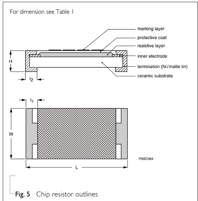
Fig. 5 Chip resistor outlines
