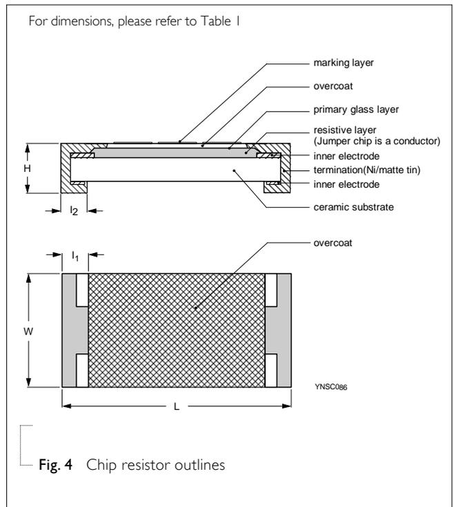
Fig. 4 Chip resistor outlines
